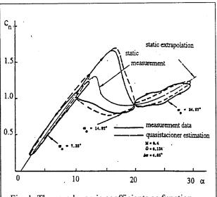
Fig. 1. The aerodynamic coefficients as function of angle of attack
