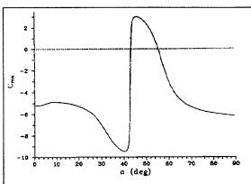
Fig.3. Pitching moment derivatives as function of AoA
