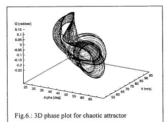
So, the our investigation gave the very interesting conclusion, the closed deterministic system (11) - (14) can result to the chaos. The chaotic motions appeared at the different frequency of excitation depend on the applied types of the aerodynamic models, but have not fundamental sensitivity to the changes in the values of the
