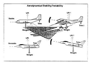
Although the aircraft becomes aerodynamically stable in supersonic flight, the centre of pressure is still further forward than for a subsonically stable design. The advantage of reduced trim drag and better turn performance is therefore still retained in supersonic flight. However, artificial stabilisation requires more effort in the design of the Flight Control System, in control law design and in final clearance work.
