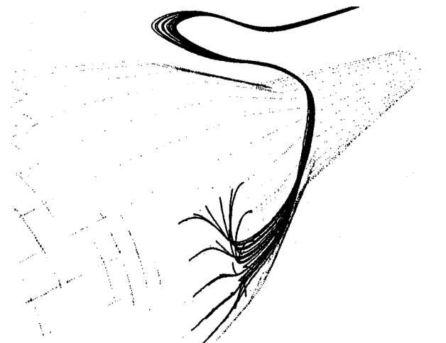
Figure 13: Particle traces showing vortex leaving the body surface on the side of the vehicle.
