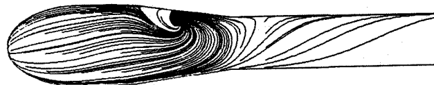
Figure 17: Side view of oil-flow lines for Atlas-Able IV configuration (computation with search up to 35th grid point).
