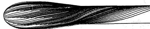
Figure 18: Side view of oil-flow lines for Atlas-Able IV payload (computation with search up to 45th grid point).
