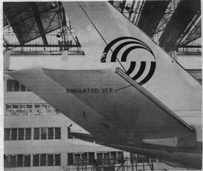
Fig. 20. Ice Ledge at Horizontal Tail
