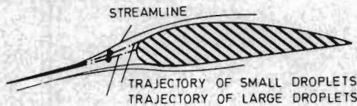
Figure 4. Deviation of Droplet Trajectories from Streamline Due to Droplet Diameter
